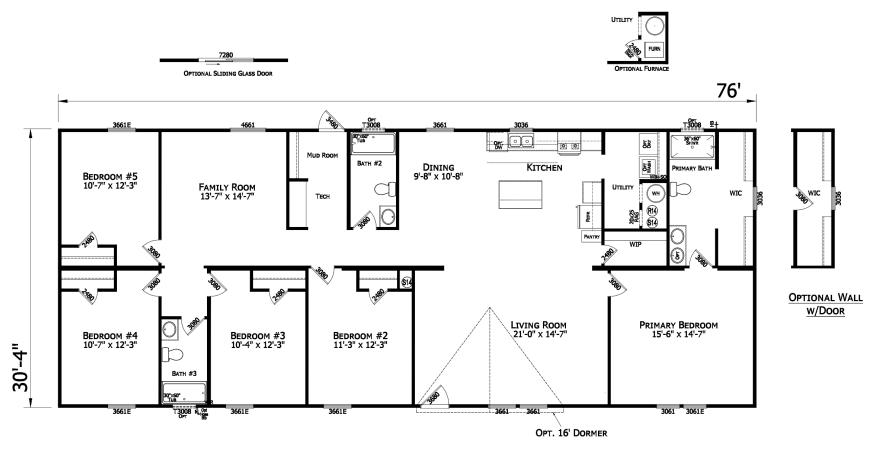
NOTE: ROOM SIZES INCLUDE WALL DIMENSIONS AND ARE NOT INDICATIVE OF TRUE NET DIMENSIONS
